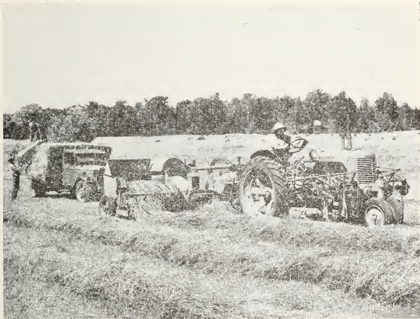
FIGURE 15.—A three-man hand-tie pickup baler baling hay. Machines of this type baled an average of 2.4 tons of hay per hour on the sample farms. Most hand-tie pickup balers are powered by a motor mounted on the baler, as is the baler here shown. Two men tie bales while the third man of the crew drives the tractor.
